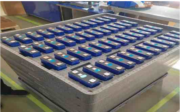
Battery cell’s collar containers + EPP foam solution
